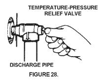
If after manually operating the valve, it fails to completely reset and continues to release water, immediately close the cold water inlet to the water heater, follow the draining instructions, and replace the temperature-pressure relief valve with a new one.
